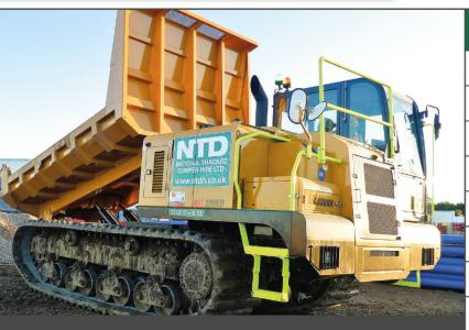
If you require a tracked dumper capable of carrying a larger volume for bulk material handling. This machine offers a carrying capacity of 11 tonne and is a popular selection on larger sites working in tandem with other machines to ensure high levels of productivity. This model is Tier 4 Final/Stage 4.
