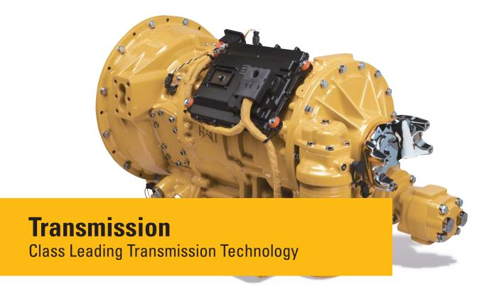
The Cat CX31 six-speed forward, single speed reverse transmission features Advanced Productivity Electronic Control Strategy (APECS) and Electronic Clutch Pressure Control (ECPC) which deliver smooth gear changes with improved acceleration and higher productivity.
