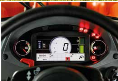
The LCD monitor shows the machine's status and settings.
