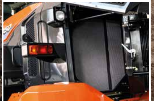
Optional anti-clogging radiators enhance durability.
