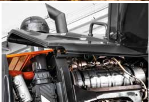
The SCR system reduces emissions.
