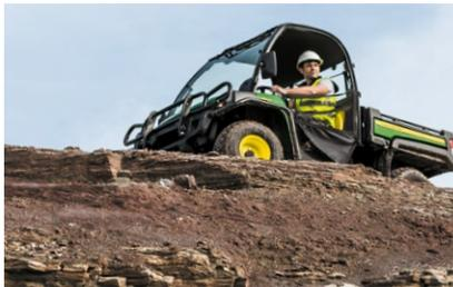
**Safety First:** Each vehicle is fitted with a ROPS (Roll Over Protection Structure) canopy and comfortable three-point seat belts to keep you safe at all times. Fully hydraulic brakes ensure first-class braking performance.
