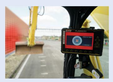
**Height Restrictions:** In situations where the excavator is in danger of hitting an overhead obstruction, such as power lines or a gantry, these can be quickly created or imported as avoidance zones from the cabin controls. Once the system is triggered, the hydraulic functions of the excavator can be slowed down or even brought to an entire stop.
