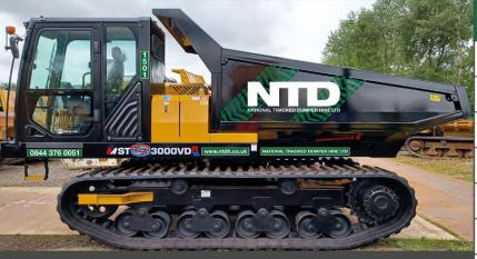
The Morooka MST 3000VDR is one of our largest tracked dumpers with an impressive 15000 kg payload. This machine is a real workhorse with a rotatable dump bed for precision work. The upper structure rotates a full 360°, so you can deliver your load where you need it and return without spinning the undercarriage.
